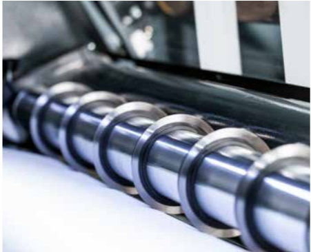
Scissor cut For best quality with long service life.
